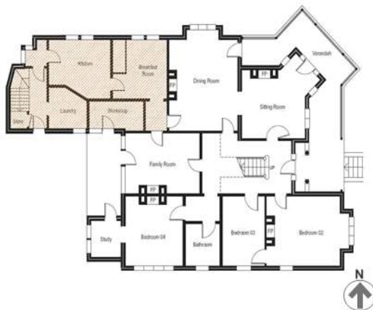
Figure 2.25 Ground Floor Plan in 2012. The 1950s alterations and additions to Sunny Brae are shown shaded. Source: David White Architects, 2020.
