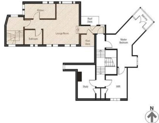
Figure 2.26 Upper Floor plan in 2012. The 1950s alterations and additions to Sunny Brae are shown shaded. Source: David White Architects, 2020.
