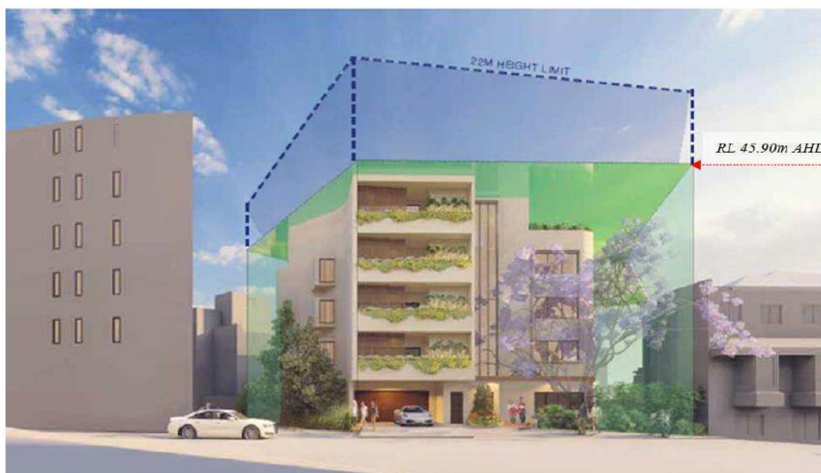
Figure 1 Proposed building envelope with the 22m maximum height control shown in dashed lines and secondary height plane of RL 45.90m AHD shown in green (source: Planning proposal)
