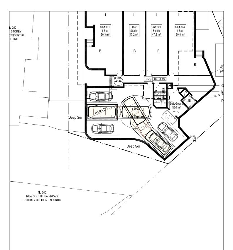
This drawing has been prepared using vehicle modelling computer software AutoTrack V5.00a in conjunction with AutoCAD 2013. The vehicle used is based upon vehicle data provided by Austroads and incorporates a reasonable degree of tolerance. However, it is not possible to account for all vehicle types/characteristics and/or driver ability.
