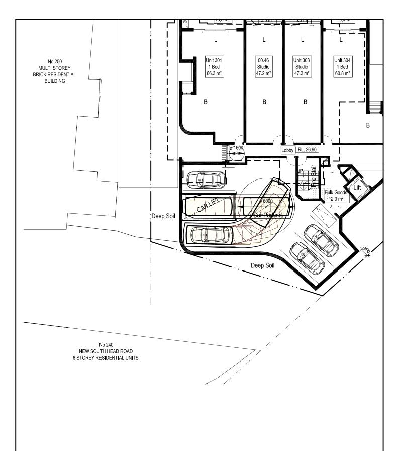
This drawing has been prepared using vehicle modelling computer software AutoTrack V5.00a in conjunction with AutoCAD 2013. The vehicle used is based upon vehicle data provided by Austroads and incorporates a reasonable degree of tolerance. However, it is not possible to account for all vehicle types/characteristics and/or driver ability.
