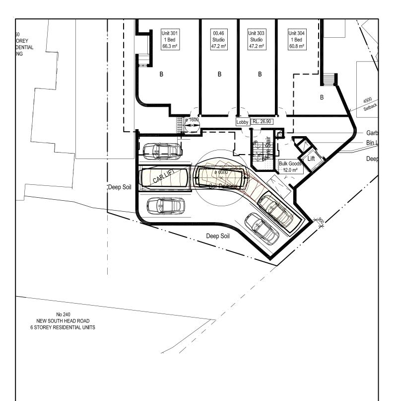
This drawing has been prepared using vehicle modelling computer software AutoTrack V5.00a in conjunction with AutoCAD 2013. The vehicle used is based upon vehicle data provided by Austroads and incorporates a reasonable degree of tolerance. However, it is not possible to account for all vehicle types/characteristics and/or driver ability.
