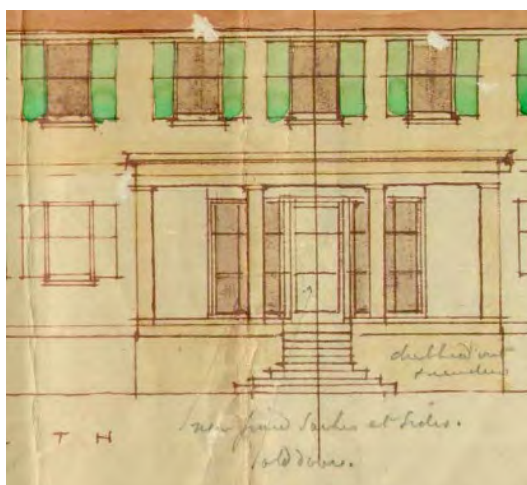
Figure 12 Extract from BA3/1939 for 43 Latimer Road, Bellevue Hill. Note the notation (far bottom) on the entrance “old door” which exemplifies Wilkinson’s approach to salvage building materials.
