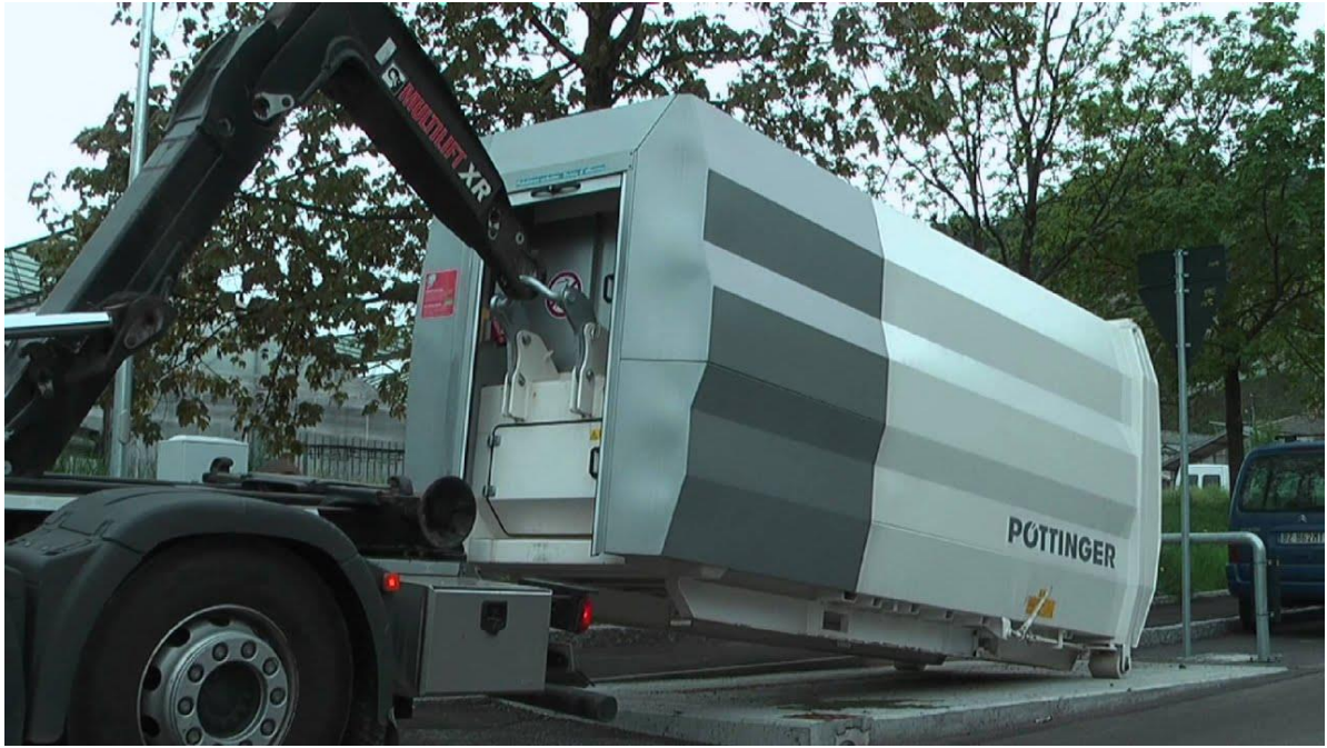
Figure 5-9: Single Axle Hook Lift Smart Compactor Hub Removal
