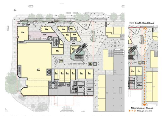
Figure 31 – Ground floor plan identifying the transport interchange entrance and through-site link Source: FJMT & Ethos Urban
