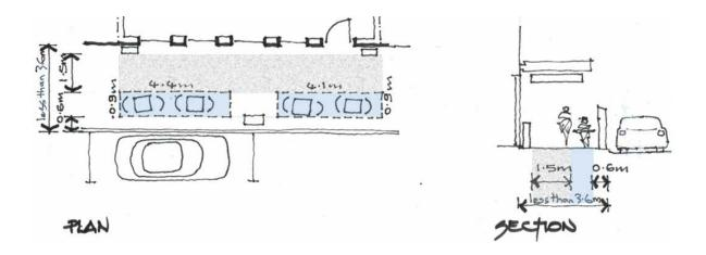
Note: This is a narrower footway (1.5 m wide), this plan can also apply to a 1.8m wide footway space.
